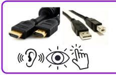
Additionally, the ActivPanel 9 Premium can be connected using an HDMI and USB touch cord. This type of connection enables audio and visual from the connected device, as well as touch capability. Please note: the cords must be plugged in to corresponding ports.
